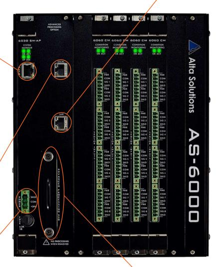
LEVERAGE OFF-THE-SHELF POWER SUPPLIES Normal +24Vdc Power (+18Vdc to +30Vdc Range)
