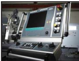
INTERFACES TO GRINDER CONTROLS Traverse, Depth of Cut, Overlap Ratio, Wheel Diameter, Roll Diameter
