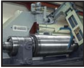
VIBRATION AND SPEED SENSORS Headstock and Tailstock Vibration, Grinding Wheel Vibration, Roll Speed, Wheel Speed
