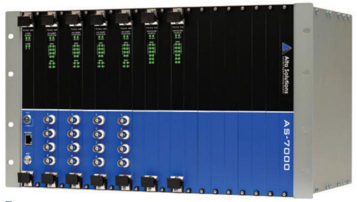
The AS-7000 can capture up to 64 dynamic signals using two 24-bit analog-to-digital converters per channel.
